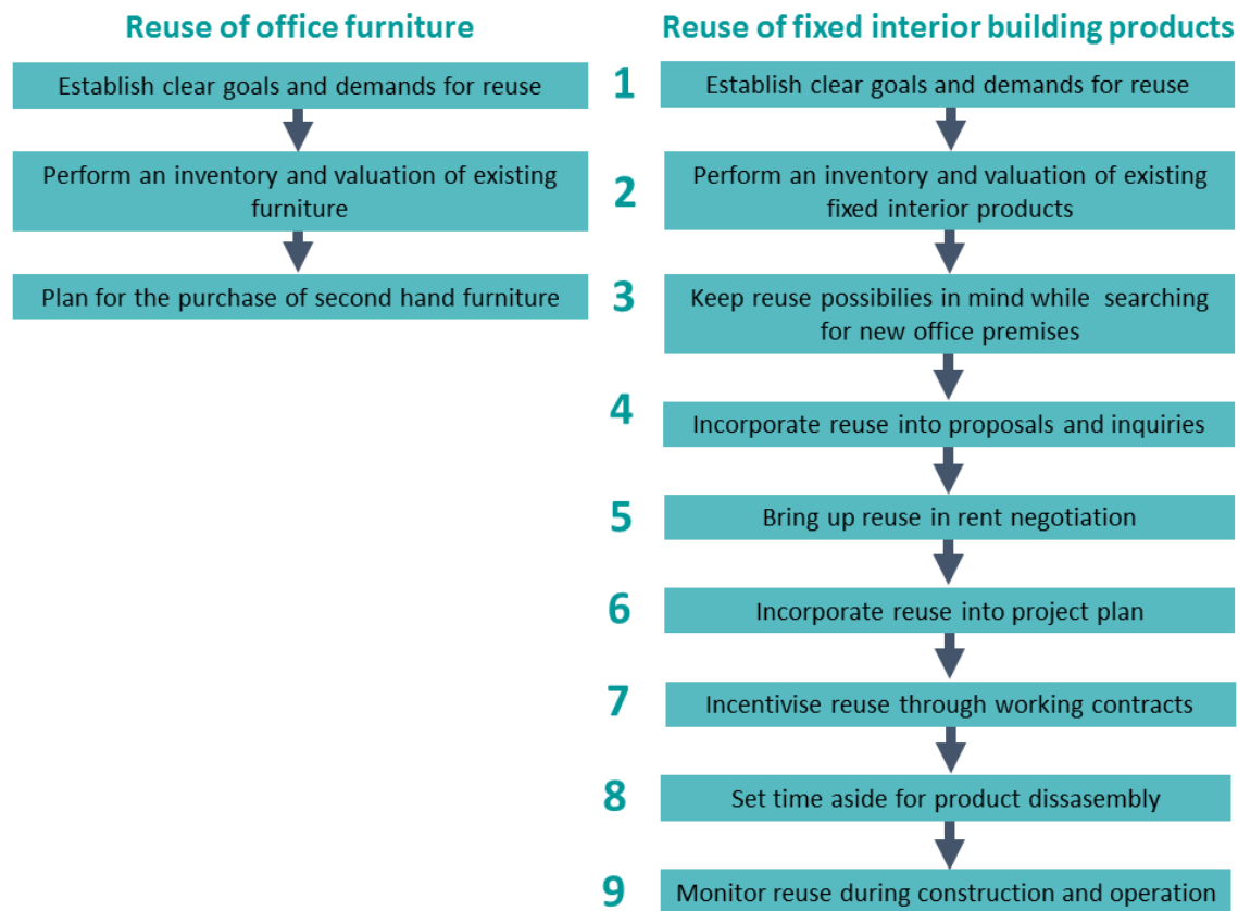
Figure 1. Working guide for reuse of furniture and fixed interior building products in relation to the renovation of office premises.
