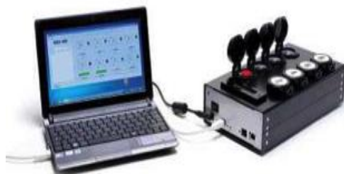
Fig 4. MBS for rapid detection of microorganisms.
