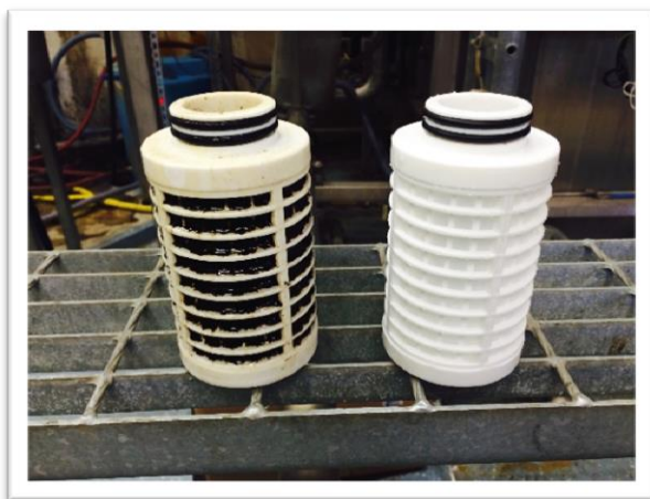
Fig D. Observation of used and new pre-filter attached in the WQM-100. [Left – clogged pre-filter in WQM-100; Right – New pre-filter before installation with MBR A effluent]. These clogged contaminants/micro-contaminants are normally not visible to the naked eye but can be observed in a filter.
