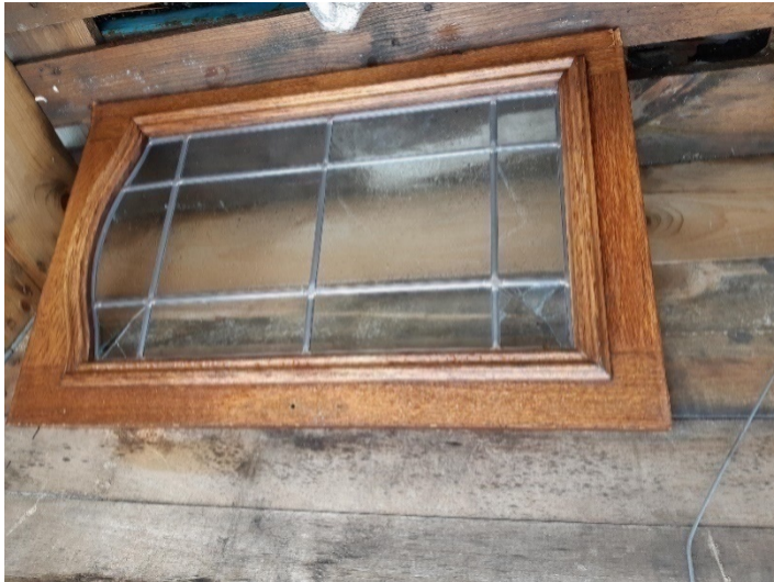
Figure 6. The armoire frame from the 50's containing lead. The product should be treated as hazardous. Ref: IVL
