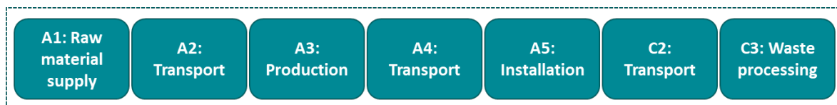
Figure 5: Overview of the considered stages in the life cycle of a multilayer parquet.
