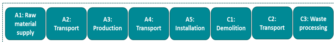
Figure 6: Overview of the considered stages in the life cycle of a PVC flooring.
