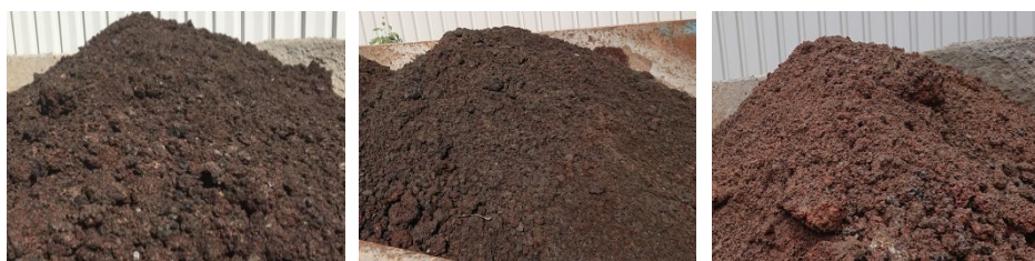
Figur 5-5 Bottenaska: (a)Borlänge slam/RT (b)Falun slam/RT (c)Mora slam
