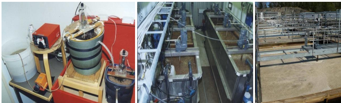
Figure 1.4. Used deammonification systems at Himmerfjärdsverket, from lab-scale over pilot-scale to full-scale treatment of supernatant.
