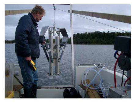
Figure 1-12 The Gemini core sampler ready to be launched from Research Vessel Perca.
