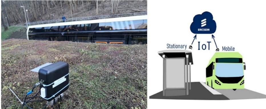
Figure 22. Implementation of low-cost particulate matter sensors as mobile and stationary units in the City of Gothenburg.
