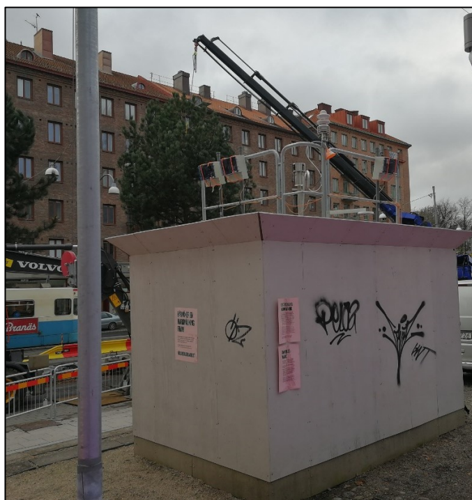
Figure 9. LoV-IoT air quality sensor platforms evaluated at the Korsvägen infrastructure project in Gothenburg.
