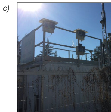
Figure 1. Comparative measurements at reference stations for validation purpose at the a) Gothenburg, Femman urban background station, b) Gothenburg, Korsvägen traffic-oriented site and c) in Santiago, Chile.
