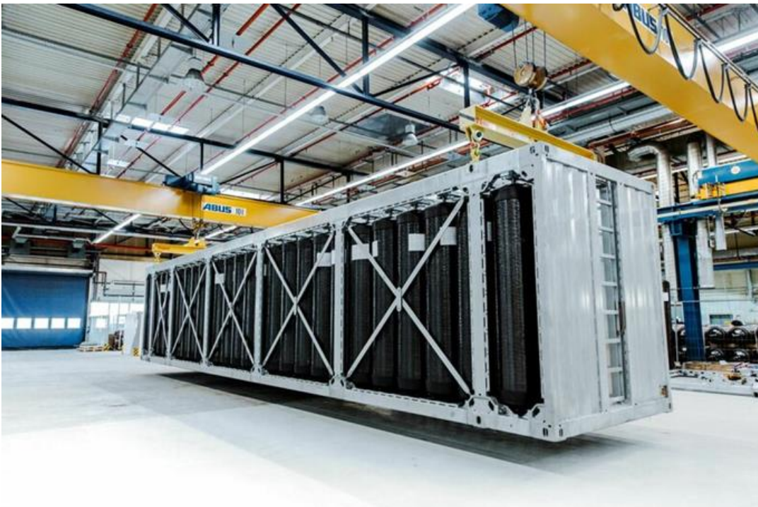
Figure 6.3 - Arrangement of pressure cylinder in 45' container. Ref.: https://hexagongroup.com/companies/hexagon-purus
