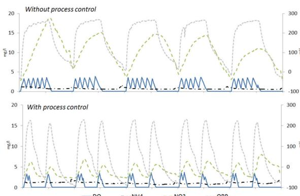
Figure 1: Basin data before and after upgrade to the process control at Green Lake
